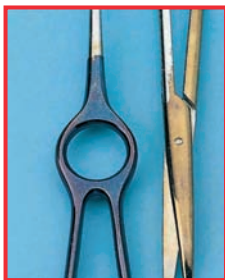
Instrumente decolorate de acid silicic
